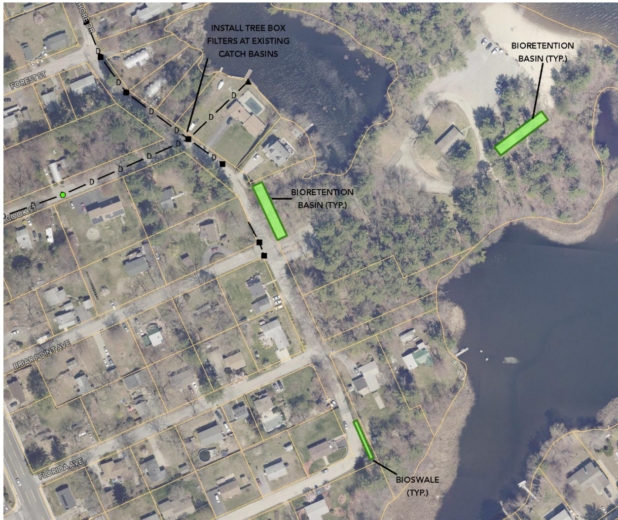
Figure 14: Potential GSI retrofit options within the ROW and on Town property near Briar Point Beach. An unmapped paved swale discharges surface flow from the southeast corner of West Shore Drive directly to Tiogue Lake
