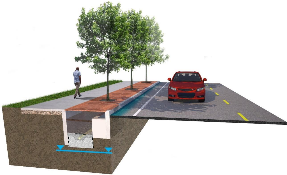
Tree box filters next to roadway
