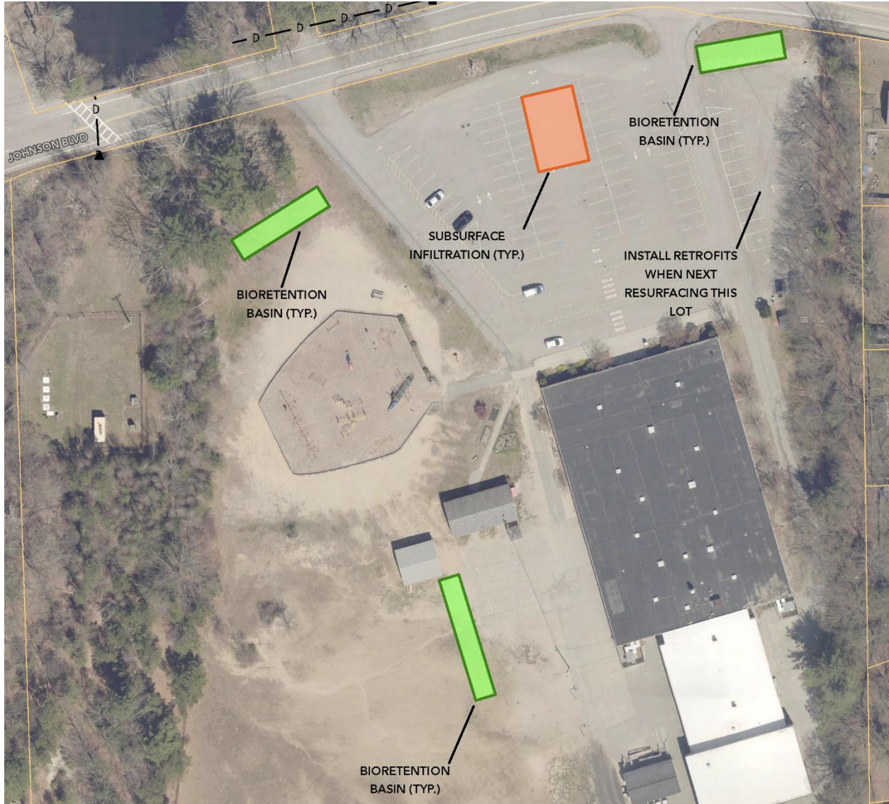
Figure 12: Potential GSI options at Hopkins Hill Elementary School. Aerial imagery and site visits indicate that channelized flow from the playground and impervious area near the pavilion discharges to a direct tributary of Tiogue Lake
