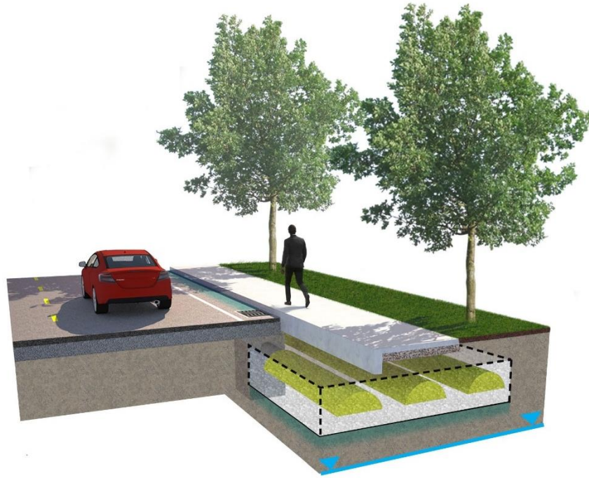
Figure 18: Subsurface infiltration chambers beneath sidewalk
